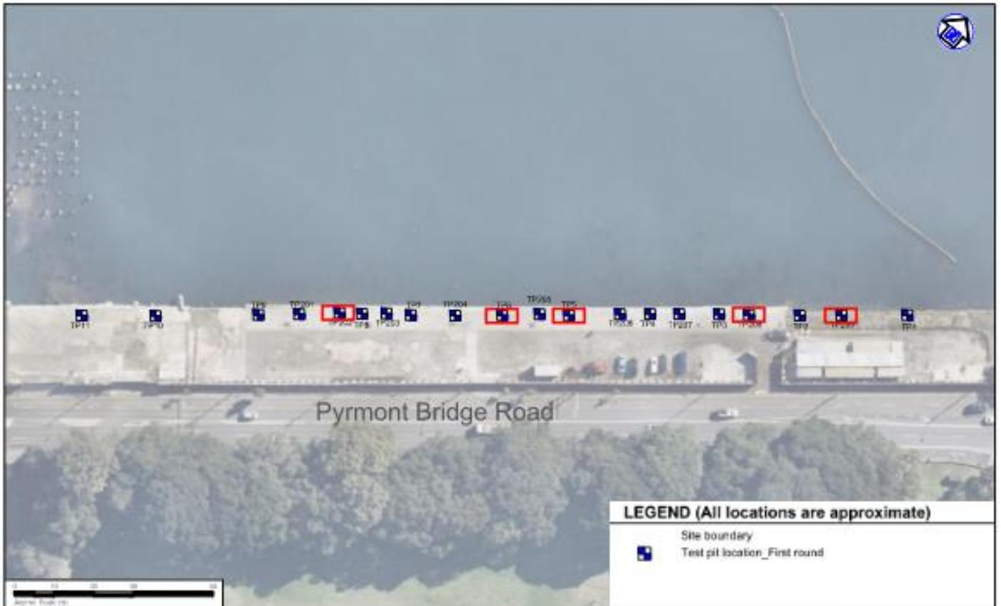
Figure 1: Test pit locations with ACM identified highlighted in red.
